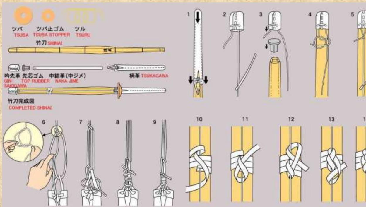
Now you should examine your shinai before and after each use. Look for busted strings, damaged leather, splinters (sand them off), cracks (wood glue and clamp and once dry, sand) and breaks (discontinue use!) Now you can keep an old shinai for spare parts as long as they are still in good condition.
